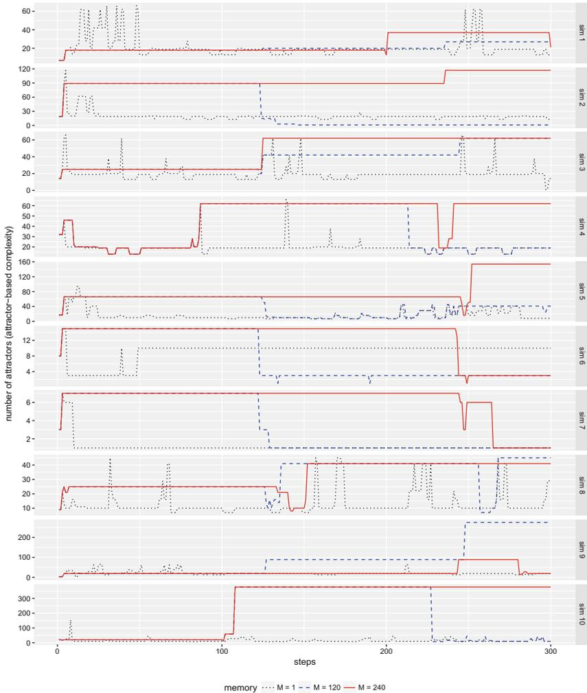
**Fig. 3.** Results of 10 simulations representing the variations of the attractor-based complexity of the BGT network over time. For each simulation, the weight matrix of the BGT network is initially randomly jittered. Then, the network is subjected to a random input stream and its attractor based complexity computed at each time step. The results for the network memory  $M = 1, 120, 240$  are represented.
