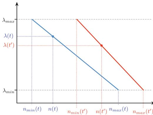
**Fig. 2.** Computation of the adaptive learning rate  $\lambda(\cdot)$  at two different time steps  $t$  (blue construction) and  $t'$  (red construction). The rate  $\lambda(\cdot)$  is defined as the image of  $n(\cdot)$  by the linear interpolation between the two points  $(n_{min}(\cdot), \lambda_{max})$  and  $(n_{max}(\cdot), \lambda_{min})$ . (Color figure online)
