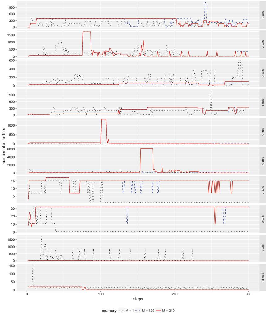
**Fig. 4.** Results of 10 simulations representing the variations of the attractor-based complexity of the BGT network over time. In this case, the network is subjected to a targeted adaptive STDP rule where constant  $C = 5$  for the three weights (Thalamus, STN), (GPe, STN) and CCortex, STN) and  $C = 1$  for all other weights (cf. Eq. 1). The results for the network memory  $M = 1, 120, 240$  are represented.
